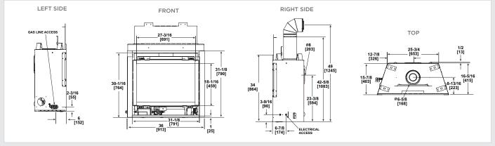
Dimensions above are in inches. Reference dimensions only. We recommend measuring individual units at installation. Assumes the use of 1/2" Sheetrock. NOTE: Combustible material should not be installed over the face. Make sure you do NOT cover the decorative door opening.
